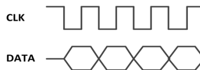
Fig. 4-24 the output data is phase aligned with the output clock
