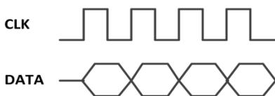
Fig. 4-24 the output data is phase aligned with the output clock
